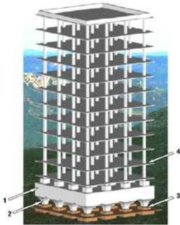
Figure 2. Elevated Building Foundation.
