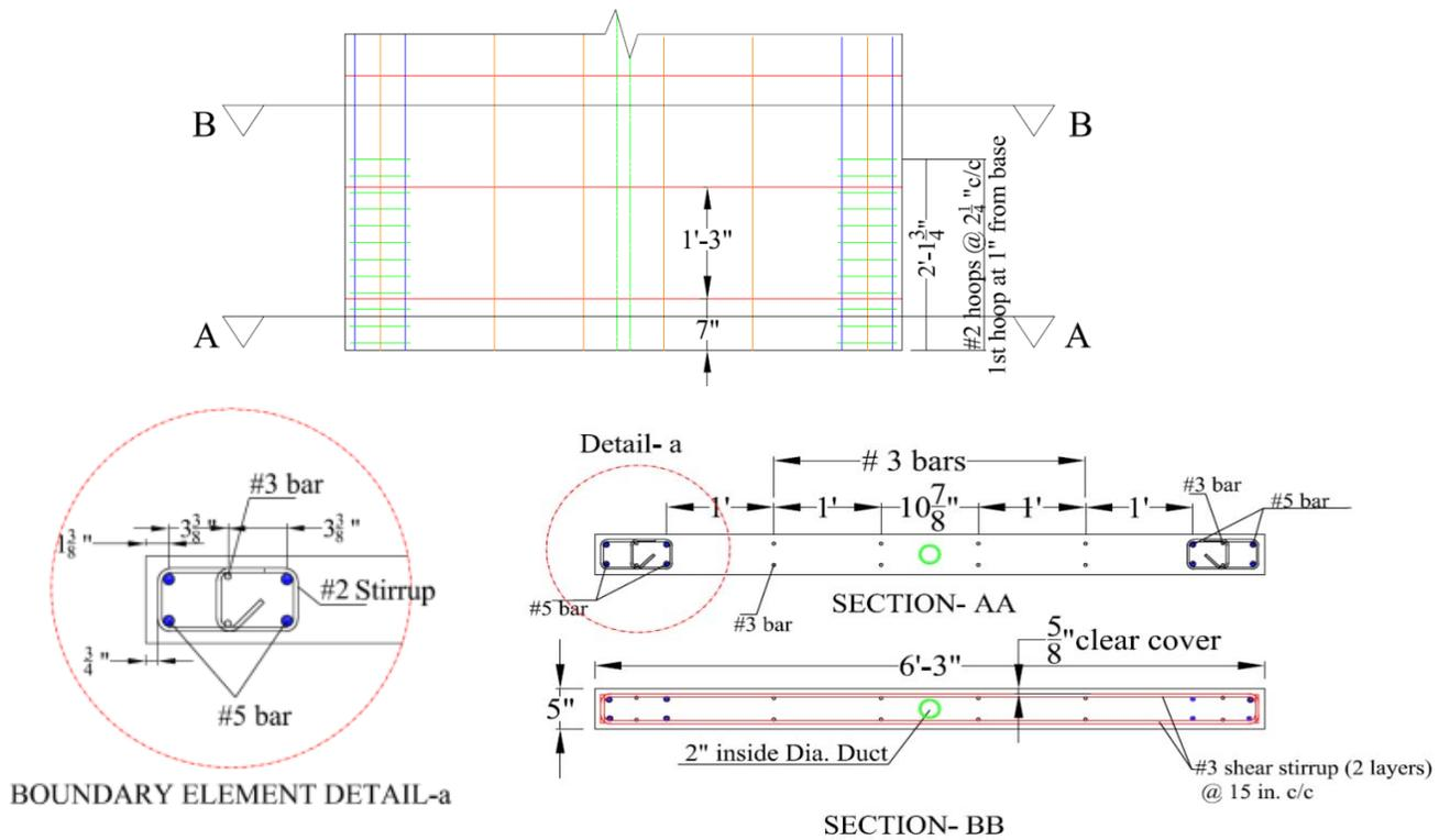
Figure 1. Typical cross-sectional details of all four walls (SRW1-4).
