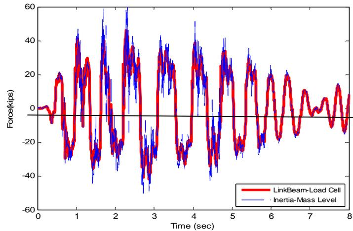
Figure 3. Inertia and link beam Force (Experimental Data) - SRW3-Kobe EQ.
