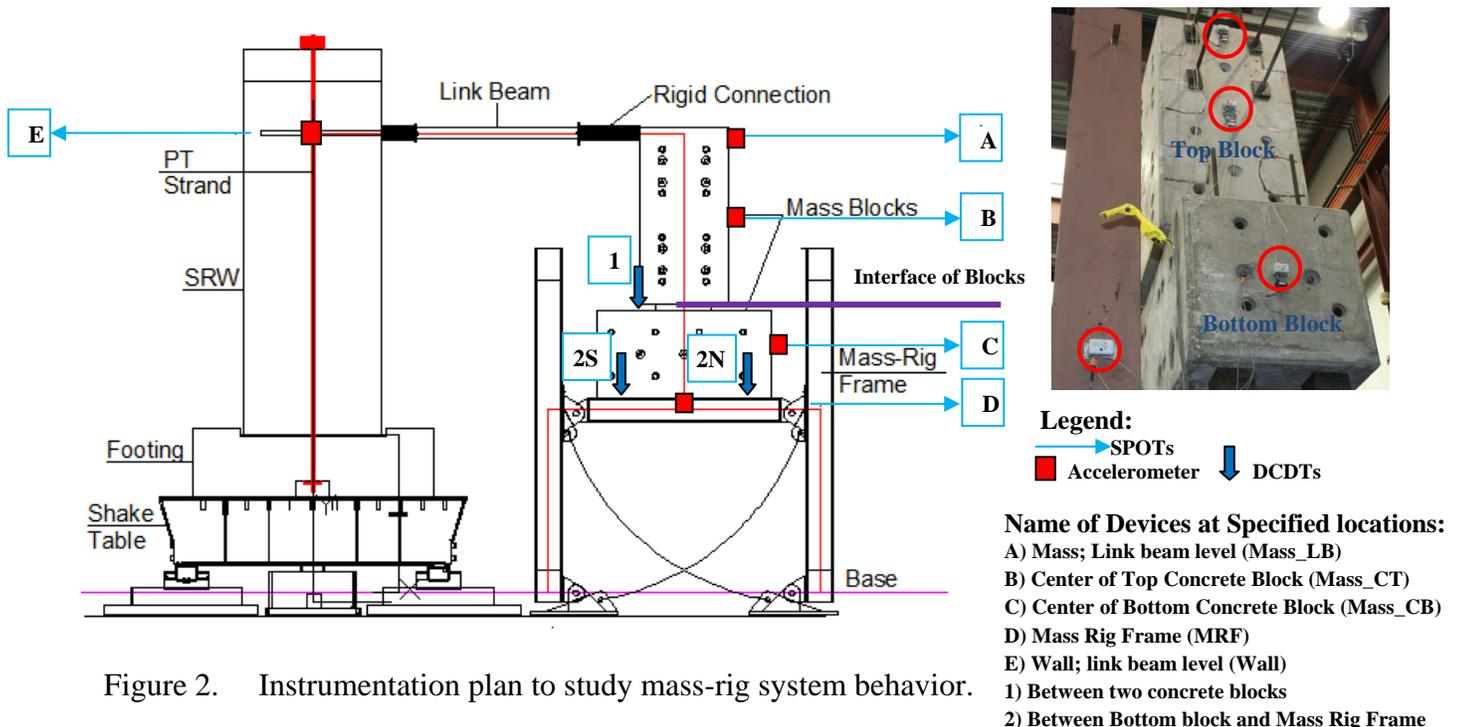
Figure 2. Instrumentation plan to study mass-rig system behavior.
